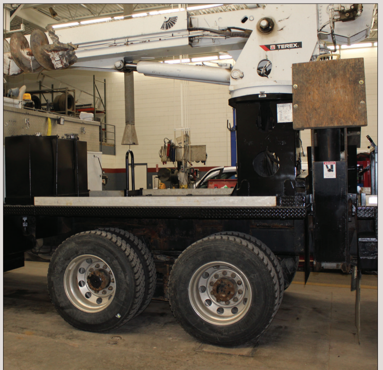
Before and after photos of the bed MVEC's mechanics replaced on a 2014 digger truck. The co-op recently decided to restore the otherwise healthy truck rather than replace it with a new one.
